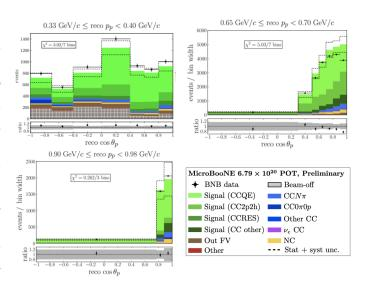
**Figure 1:** Selected CCNP events as a function of  $cos(\theta_p)$  in different regions of leading proton reconstructed momentum.
