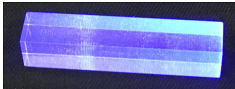
Figure 2: Left: the 3D printed scintillator bar with dimensions of 10 \times 10 \times 50 \text{ mm}^3 exposed to UV light. This sample is used to evaluate the attenuation length of 3D printed scintillator. Right: Light output as a function of the ^{90}\text{Sr} \beta -source distance to SiPM.
