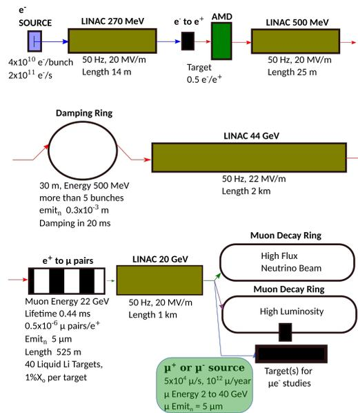
Figure 1: Low emittance muon beam production
