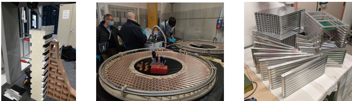
Figure 2: Crystal piling up test on a CMM ( left ). Back Plate leak test at Cinel, Vigonza (Italy) ( center ). Preparation of the create sides for the leak test at INFN Laboratories in Pisa, Italy ( right ).
