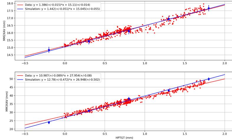
**Figure 3:** Horizontal muon beam centroid position at MM2 and MM3 as a function of the horizontal position of the proton beam on target: measurement data (red dots and fitted line) and simulation (blue line).
