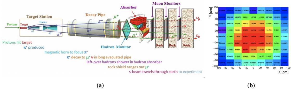
**Figure 1:** (a) Schematics of the NuMI beamline. (b) 81 pixels of signal readout at MM1. The numbers in pixels are the voltage signal.
