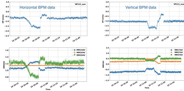
**Figure 2:** NuMI beam position on target scan data. Left: horizontal scan, right: vertical scan. Top row: beam position on target, bottom row: horizontal and vertical centroids of the muon beam at MM1 (blue), MM2 (orange), and MM3 (green).
