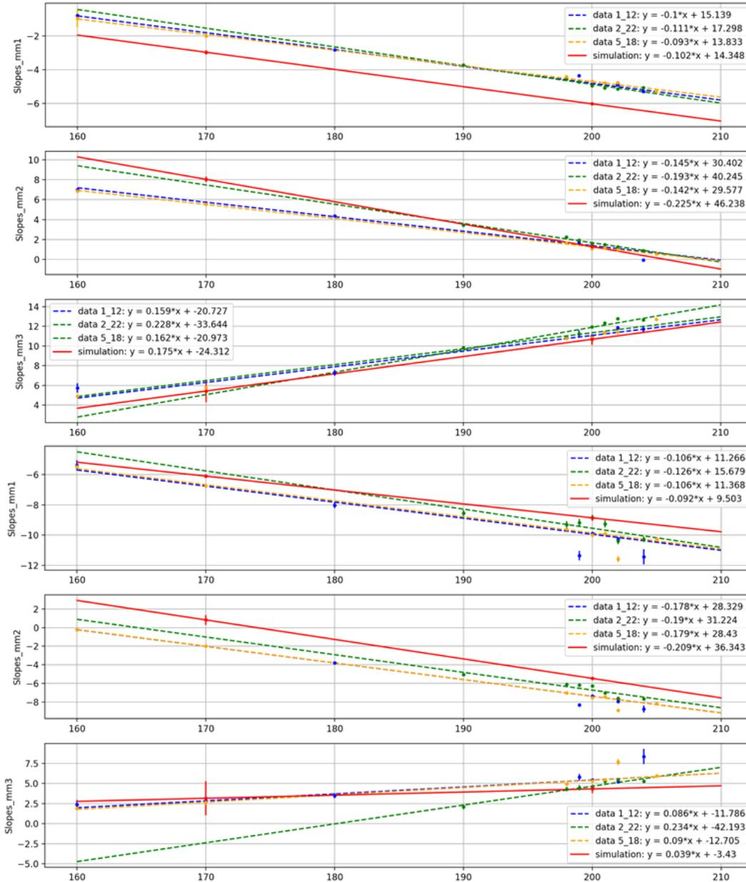
**Figure 5:** Slope of the line characterizing muon beam horizontal (vertical) position dependence on the proton beam horizontal (vertical) position as a function of horn current. Solid red line: simulation result, blue dashed line: Jan 12, 2021 horn current scan, green dashed line: Feb 22, 2021 horn current scan, yellow dashed line: May 18, 2021 horn current scan.
