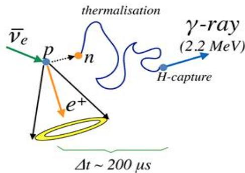
Figure 1. Hydrogen thermalisation of neutrons
