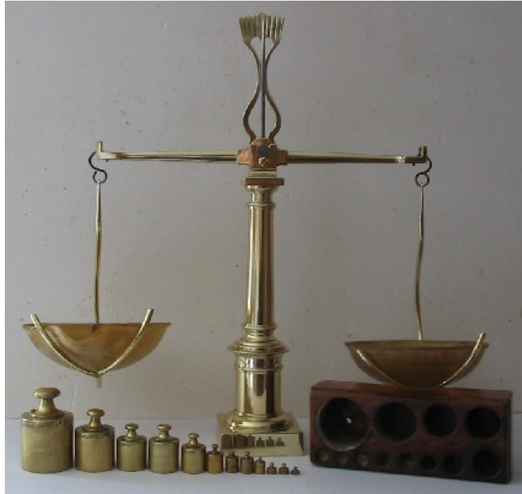
Figure 4: A two-arms scale. Objects to be weighted can be placed on a dish, and reference weights are placed on the other to reach equilibrium.
