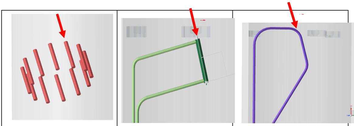
Figure 1. Three target design options. Left – rotating elements; Center – fixed granular with gas cooling; Right – “conveyor” target.
