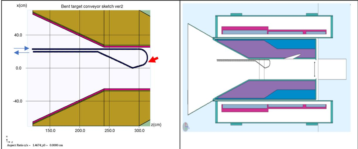
Figure 2. Simulation models of the W conveyor target. Left: MARS15. Right: FLUKA. Red arrow shows the proton beam direction. The blue arrows show the circulation flow direction.
