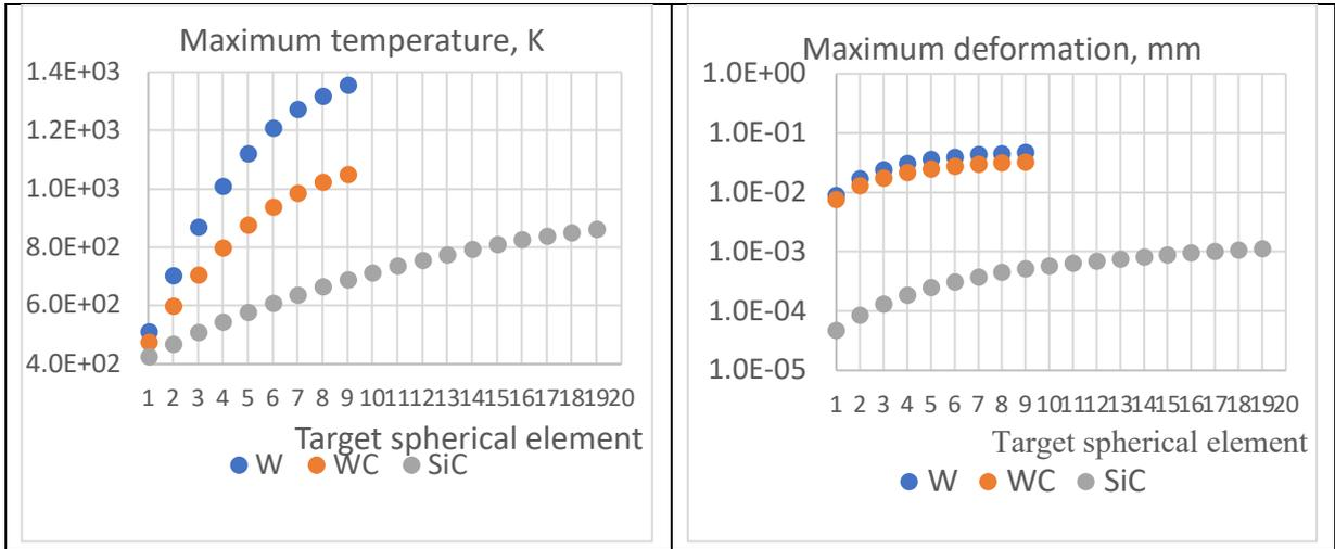
Figure 4. ANSYS analysis of the conveyor target. Left: maximum temperature in one cycle. Right: maximum mechanical deformation in one cycle.
