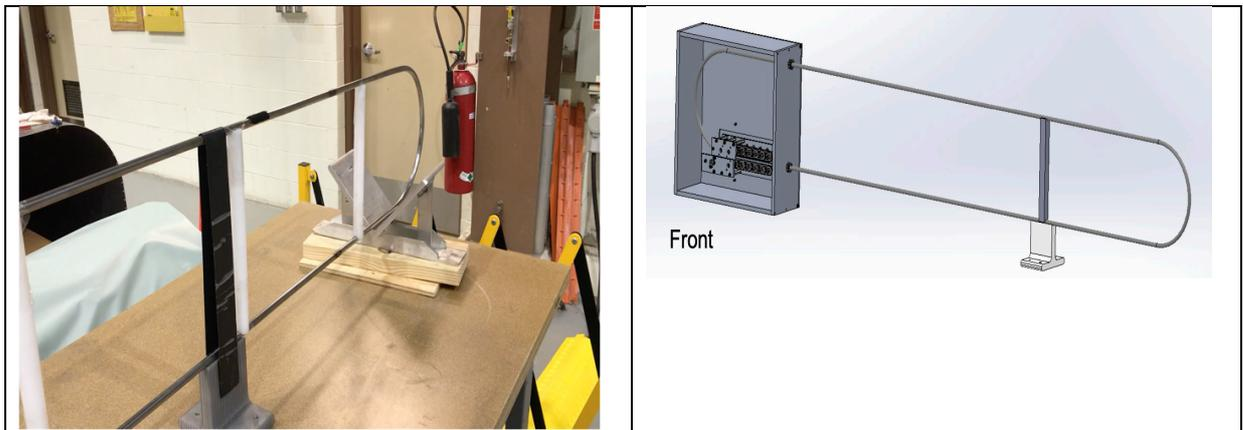
Figure 5. The first prototype of the conveyor target. Left: at Fermilab (MI-8 mezzanine). Right: a CAD model used in the fabrication.
