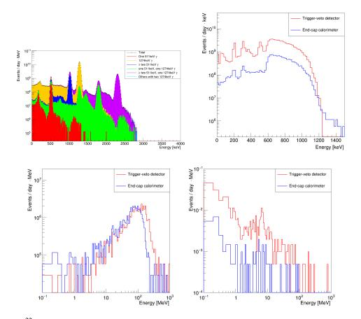
**Figure 3:** <sup>22</sup>*Na* positron source related (top left), intrinsic radioactivity from LYSO related (top right), cosmic muons, both correlated and uncorrelated (bottom left), cosmic electromagnetic particles, both correlated and uncorrelated (bottom right)
