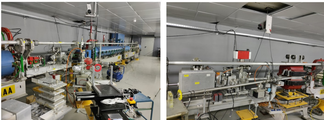
Figure 2: Beam extraction points at Linac-200: left – EP1, right – EP2.
