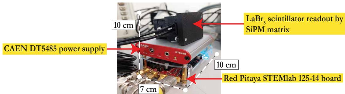
**Figure 1:** Experimental setup: from bottom to top: Red Pitaya STEMlab 125-14 board, CAEN DT5485P power supply and Ce:LaBr<sub>3</sub> scintillator readout by a  $2 \times 2$  SiPM matrix.
