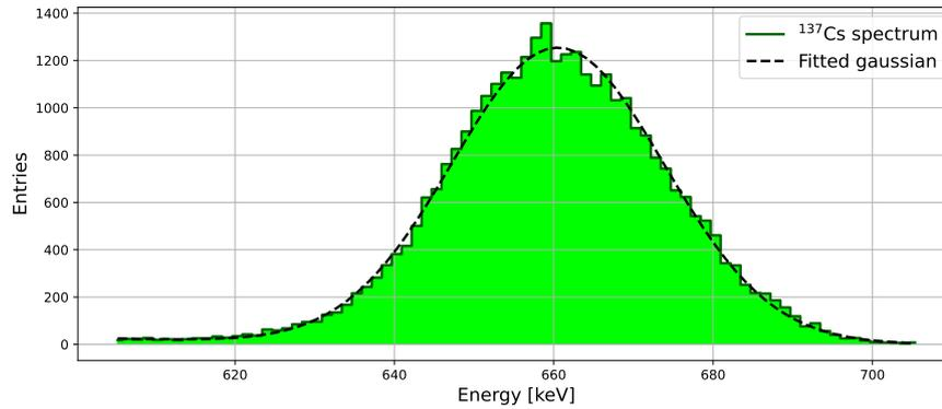
**Figure 2:** Gamma spectrum of a  $^{137}\text{Cs}$  source, acquired with  $\text{Ce:LaBr}_3$  scintillating crystal readout by a 2x2 SiPM matrix, to measure the energy resolution.
