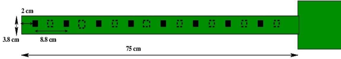
Figure 4: Hall probe sensor
