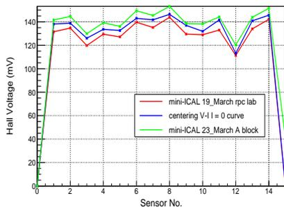
Figure 6: Offset voltage in the absent of magnetic field
