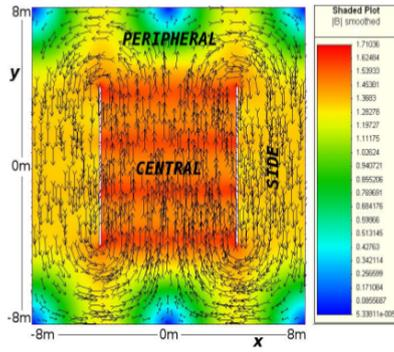
Figure 1: Magnetic field map for the ICAL
