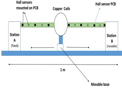
Figure 8: Calibration set up
