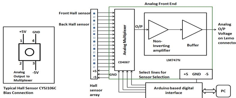
Figure 5: Schematic of the set up of Hall probe
