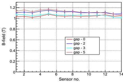
Figure 10: Magnetic field for the gap-0,2,3 and 5
