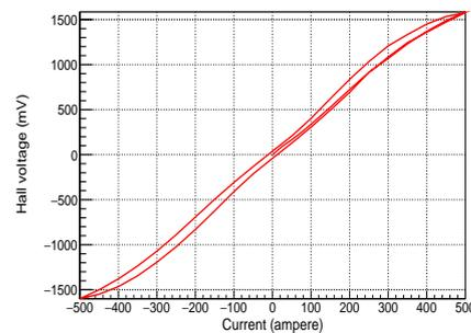
Figure 7: Hall voltage vs current after centering the V-I curve
