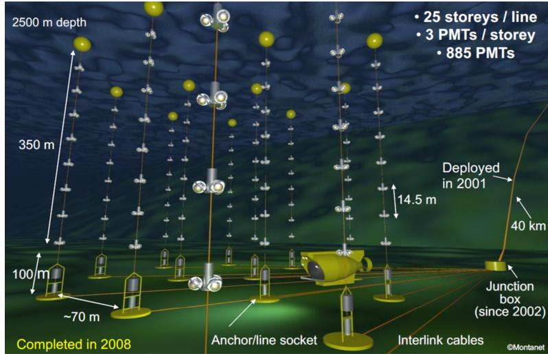
**Figure 1:** Illustrative view of the underwater detector, with 12 lines anchored at a depth of 2.5 km, 40 km off the coast of Toulon, South of France. ANTARES has been operational from 2008 to 2022.
