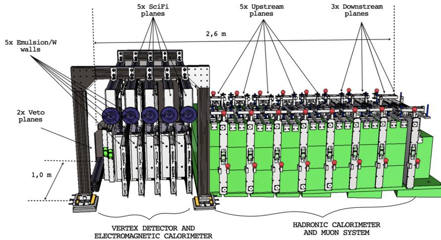
**Figure 2:** Layout of the SND@LHC detector. Particles from IP1 arrive from the left and encounter the two veto planes, the target, the hadronic calorimeter and the muon system [10].
