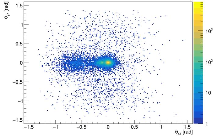
**Figure 3:** Distribution of the reconstructed muon track slopes in the SND@LHC detector. The peak around 0 corresponds to the tracks coming from the ATLAS interaction point. There are other peaks, correlated to tracks coming from machine elements in the tunnel. The tracks at higher  $|\theta_{yz}|$  are produced by cosmic rays.
