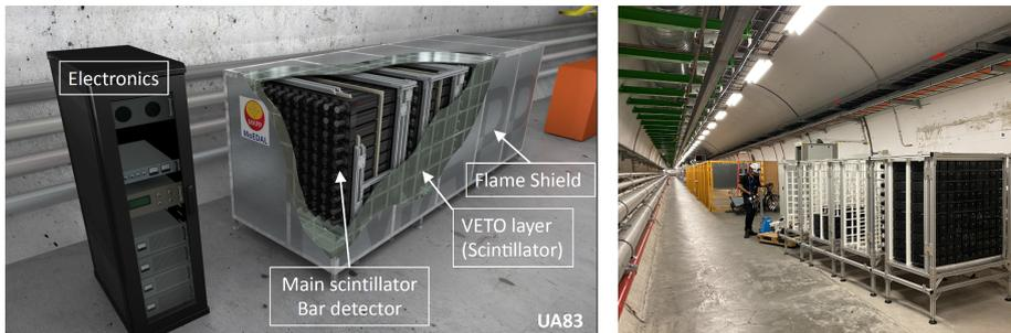
**Figure 3:** (Left) The MAPP-1 detector; (Right) The installation of MAPP-1 in the UA83.
