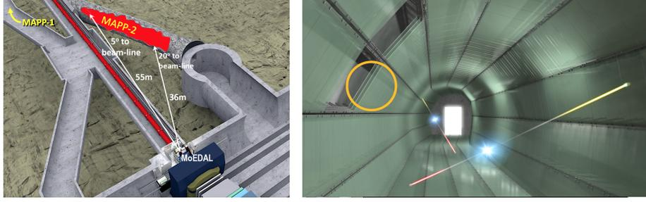
**Figure 5:** (Left) The disposition of the MAPP-2 detector in the UGC1 gallery. (Right) A 3D depiction of part of the MAPP-2 detector fiducial volume in the UGC1 gallery lined with 3 layers of large scintillator tiles with fine grain (1 cm pitch) WLS fibre readout in X-Y .
