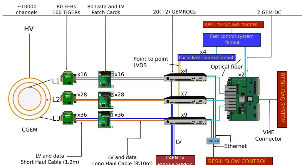
**Figure 1:** Complete scheme of the CGEM-IT readout chain [5]
