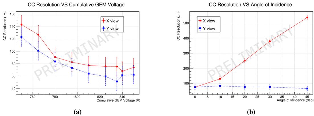
**Figure 4:** Behavior of the spatial resolution as a function of the cumulative voltage applied to the GEM electrodes at  $0^\circ$  angle of incidence, on the left, and as a function of the angle of incidence at a cumulative GEM voltage of 835 V, on the right.
