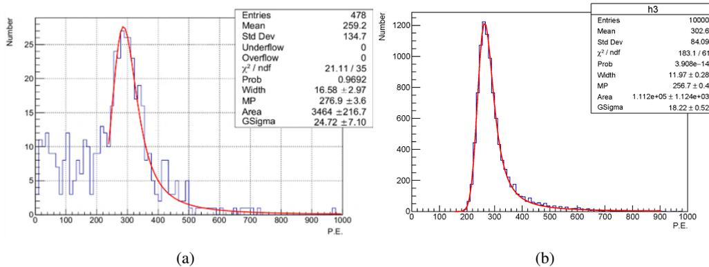
**Figure 4:** The MIP response of a scintillating glass tile: (a) cosmic ray test and (b) optical simulation.
