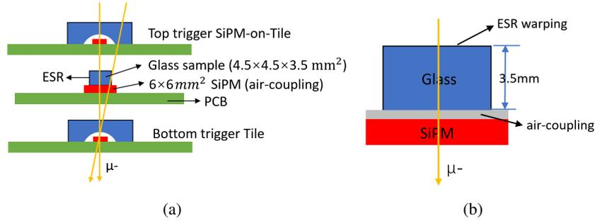
**Figure 3:** The schematic of the geometry setup: (a) cosmic ray test and (b) optical simulation.
