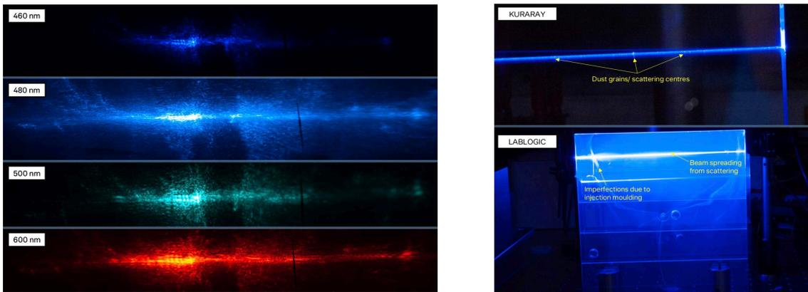
**Figure 2:** Interference observed from Mie scattering in the LabLogic WLS sample (left). Impurities, dust grains and surface inclusions in labelled samples (right).
