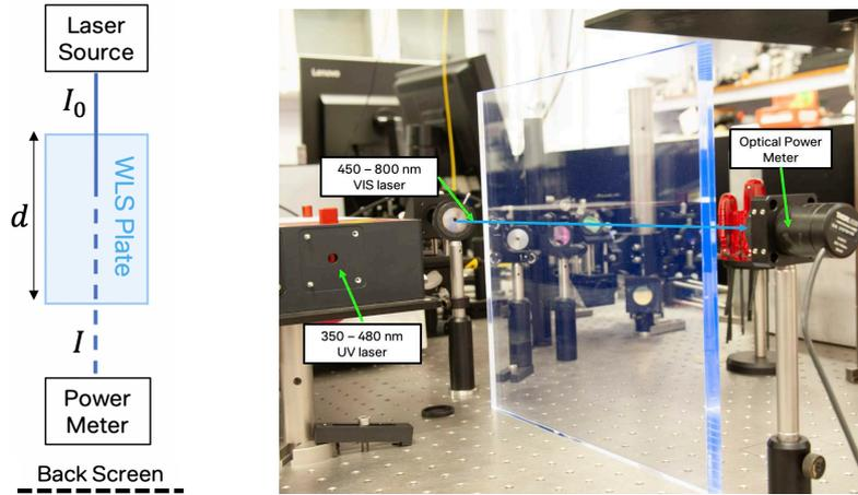
**Figure 1:** Schematic diagram of an optical measurement setup (left). Photograph of the experimental setup with a Kuraray WLS sample (right).
