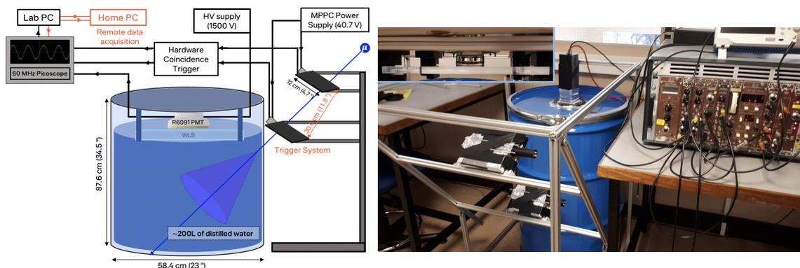
**Figure 4:** Schematic diagram (left) and photograph (right) of the Baby-K test setup.
