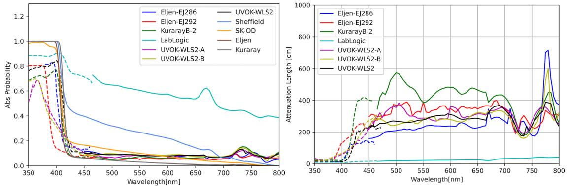
**Figure 3:** Absorbance (left) and attenuation length spectrum (right) measured as a function of wavelength for several candidate WLS samples. Measurements taken with UV laser filter (dashed) and with VIS laser filter (solid) are shown.
