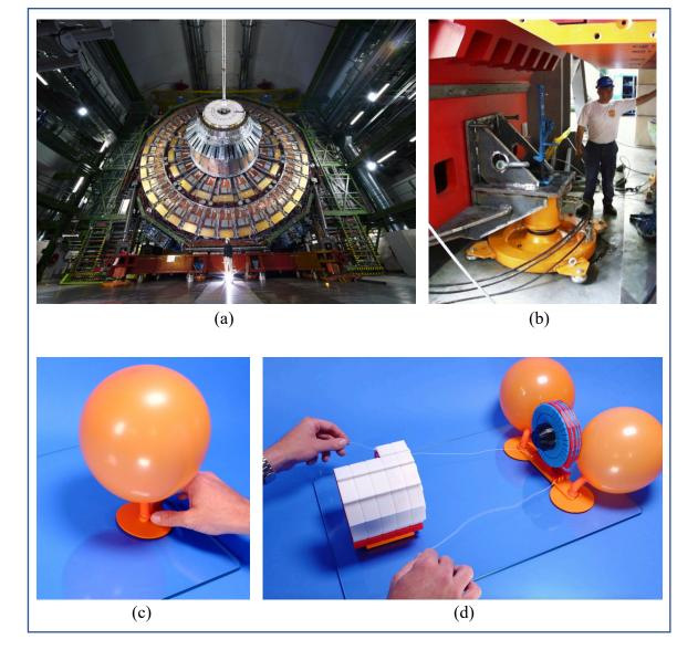
**Figure 1**: (a) Slice of CMS detector (b) Air pads (in orange) (c) 3D printed air pad for new educational activity at CERN Science Gateway (d) Alignment and closing challenge in new educational activity replicating real engineering challenge at CERN. *Image credit: CERN*.
