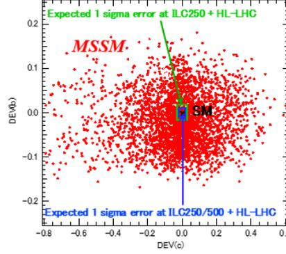
**Figure 2:** The scatter plot in the  $\text{DEV}(c)$ - $\text{DEV}(b)$  plane obtained from the MSSM parameter scan described in Section 4. "X" marks the SM point. The green and blue box indicate the expected  $1\sigma$  error at [ILC250 + HL-LHC] and [ILC250/500 + HL-LHC], respectively [6].
