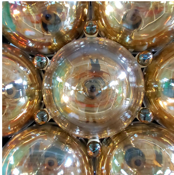
Figure 3: Installation pattern for the JUNO photomultipliers tubes.
