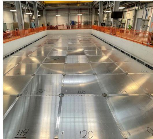
**Figure 3:** Left: illustration of the Top CRT module and its different components. Right: picture of the horizontal plane of the Top CRT system fully installed on top of the ICARUS detector.
