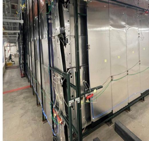
**Figure 2:** Left: picture of the Bottom CRT on the ground pit of the ICARUS cryostat. Right: picture of the south-west corner of ICARUS fully covered by the Side CRT modules.
