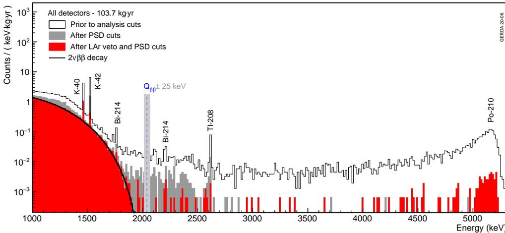
**Figure 1:** Energy distribution of GERDA Phase II events between 1.0 and 5.3 MeV before and after analysis cuts; the exposure is 103.7 kg yr. The expected distribution of  $2\nu\beta\beta$  decay events is shown assuming the half-life measured by GERDA [11]. The prominent  $\gamma$ -lines and the  $\alpha$  population around 5.2 MeV are also labeled.
