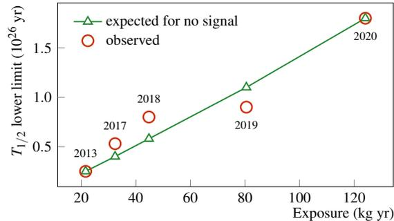
**Figure 3:** Circles: lower limit (90% C.L.) on the  $0\nu\beta\beta$  decay half-life of  $^{76}\text{Ge}$  set by GERDA as a function of the exposure [9, 13, 15, 16]. Triangles: median expectation in the assumption of no signal.
