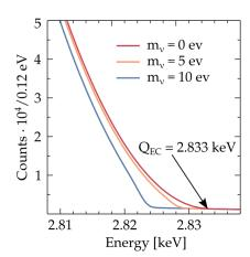
**Figure 1:** On the left, a simulation of the  $^{163}$ Ho calorimetric spectrum that assumes Q = 2.80 keV. It has been computed considering a statistics of  $10^4$  events, a pile-up fraction of  $10^{-6}$ , a FWHM resolution of 2 eV. On the right, a zoom on the endpoint region that highlights the reshaping due to a non vanishing neutrino mass.
