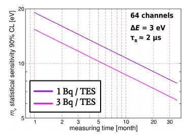
**Figure 4:** Taking into account a HOLMES low-dose measurement, this plot shows the expected upper limit assessment on  $m_{\nu}$ . The simulation involves 64 TESs with an energy resolution of 3 eV and a time resolution of 2  $\mu$ s (matching a pile-up fraction of events of  $10^{-4}$ ).
