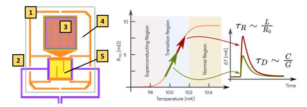
**Figure 2:** The final TES design on the left and an illustration of the TES working principles on the right. [1] is the Cu perimeter, [2] is the bias circuit, [3] is the gold absorber, [4] is the  $Si_2N_3$  substrate and [5] is the Mo/Cu sensor. In the plot, the red and the green signals are produced by two different energy depositions.
