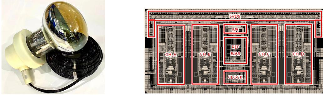
(a)  $\varnothing$ 20 cm microchannel plate photomultiplier.
