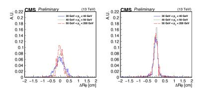
**Figure 2:** GEM demonstration [3] results to compare two propagation methodes. Residual ( $\Delta R\phi$ ) distributions for muons ( $p_T > 30 \,\text{GeV}$ ) on Layer 2 of GE1/1 superchambers 27, 28, 29, 30 (after its alignment), relative to the inner tracker (left) and the ME1/1 chambers (right) in the minus endcap for the Run-2 data. The residuals with the CSC segment back-propagation show no  $p_T$  dependence as expected.
