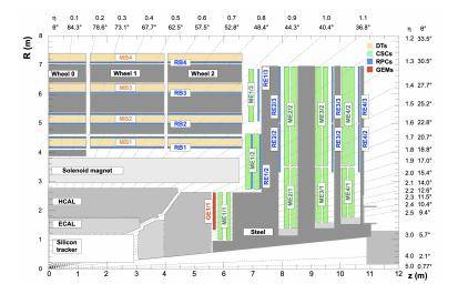
Figure 1: The CMS Muon System.
