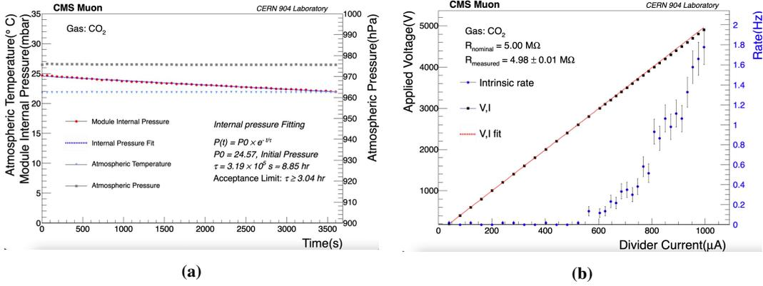
Figure 4: (a) An example of QC3 passed result, (b) QC4 passed result.
