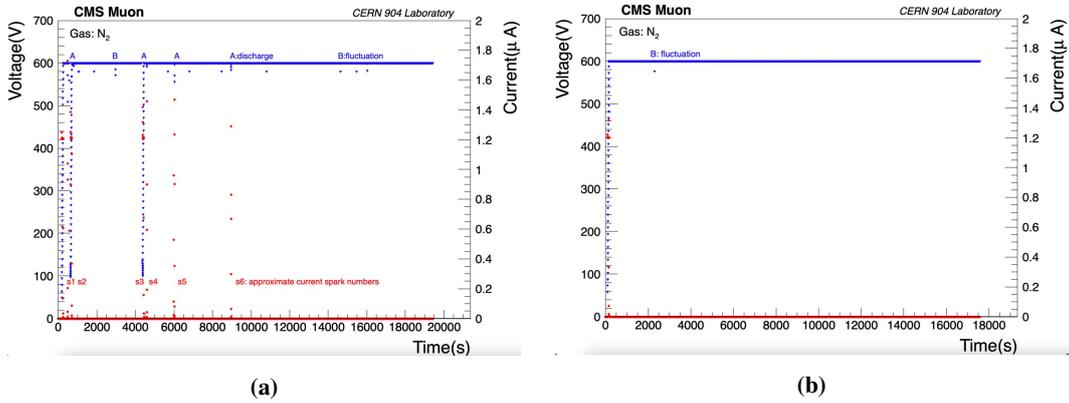
Figure 3: (a) QC2b part2 failed, (b) QC2b part2 passed.
