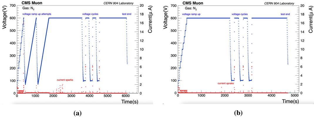
Figure 2: (a) QC2b part1 failed, (b) QC2b part1 passed.
