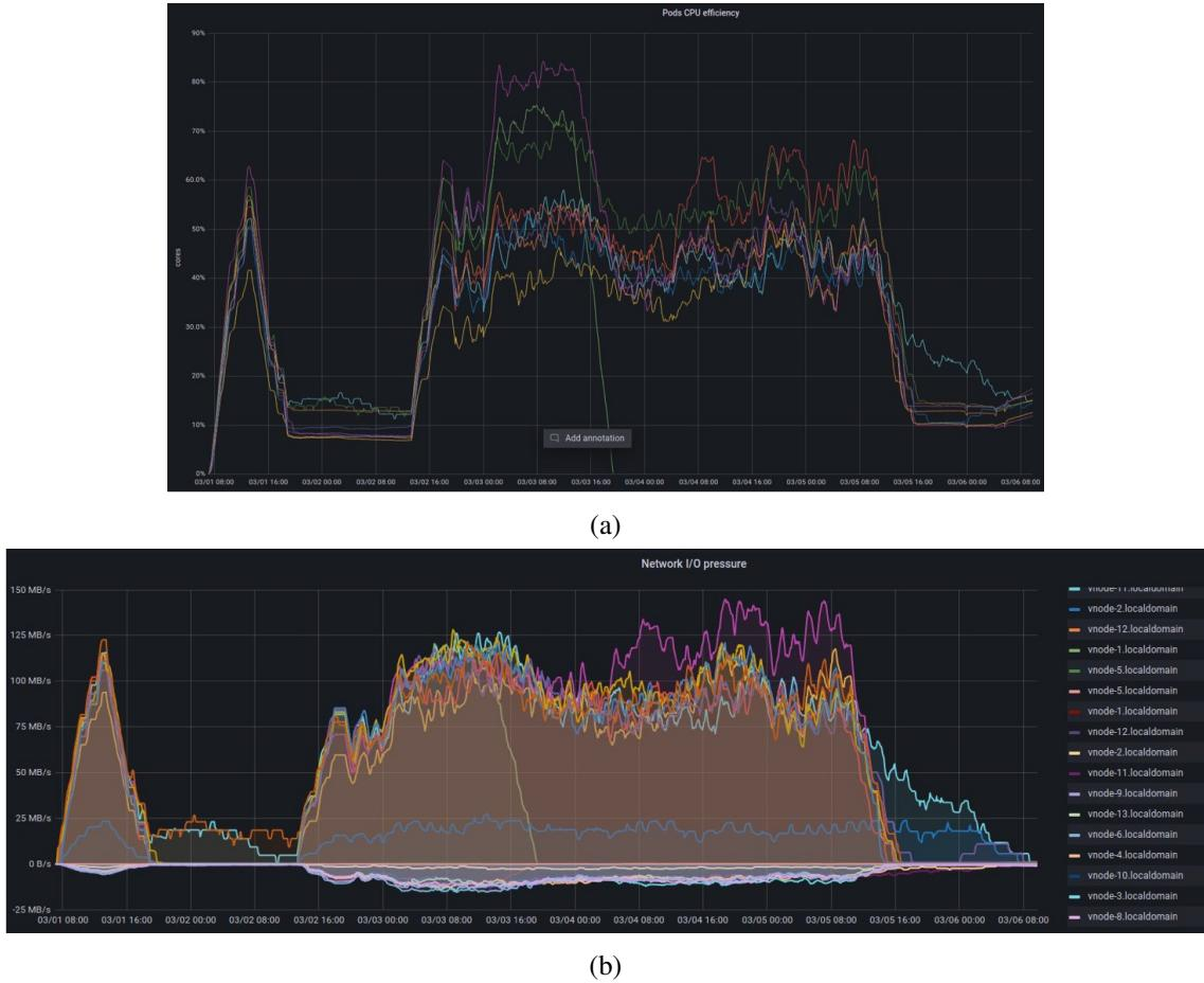
**Figure 1:** In picture (a) we can see the cpu efficiency of *Fermi* jobs. The value is referred to the first implementation and not yet optimized. Picture (b) represents the throughout generated by the worker-nodes that analyze downtime data present on the MinIO storage.
