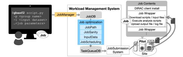
**Figure 1:** Workflow of usual analysis job submission on DC system. In the gbasf2 command, script.py shows the analysis script. Blue box shows a executor, and the job optimization is performed using four executors. Orange box and cylinder show a service and a database (DB), respectively.
