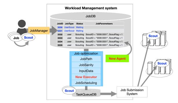
Figure 3: Design and workflow of the scout job framework
