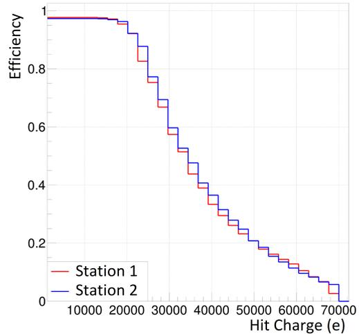
**Figure 2:** Hit reconstruction efficiency vs. reconstructed hit charge.
