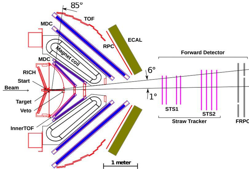
**Figure 1:** Schematic drawing of HADES and the hyperon upgrade. [3]
