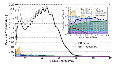
Figure 2: Visible energy spectrum and background spectra expected in JUNO detector.
