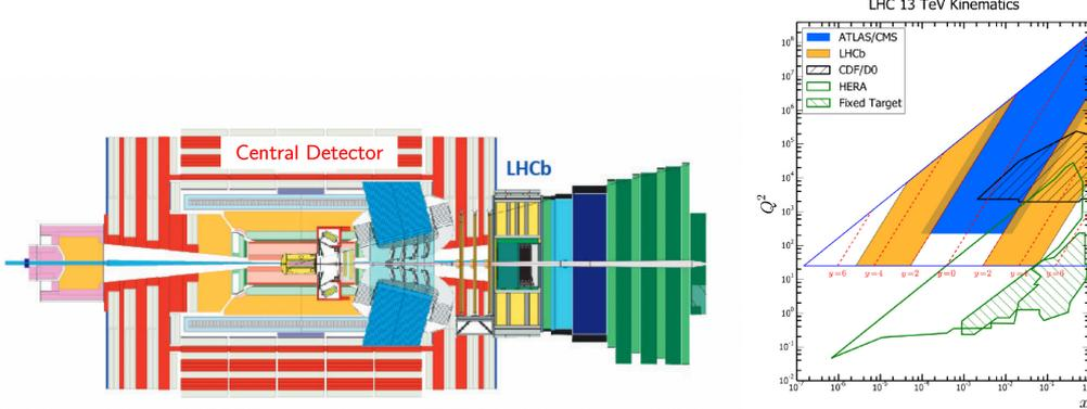
**Figure 1:** ATLAS, CMS and LHCb detector (left) and  $x - Q^2$  plane showing the acceptance of several experiments (right), where  $x$  is the longitudinal momentum fraction of the proton carried by the parton and  $Q^2$  is the energy scale of the interaction.
