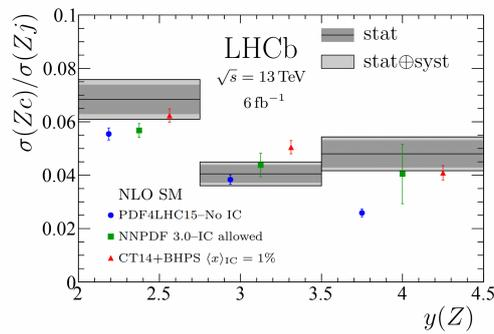
**Figure 8:** Measurements of  $\sigma(Zc)/\sigma(Zj)$  in several pseudorapidity bins, compared to NLO SM predictions.
