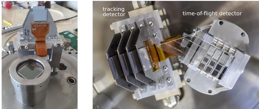
**Figure 2:** Photographs of the new ToF system with the out-of-vacuum solution. Left: photomultiplier behind the window is visible in the front, the silicon tracker in the back. Right: top view; the silicon tracker is on the left and the ToF detector on the right.
