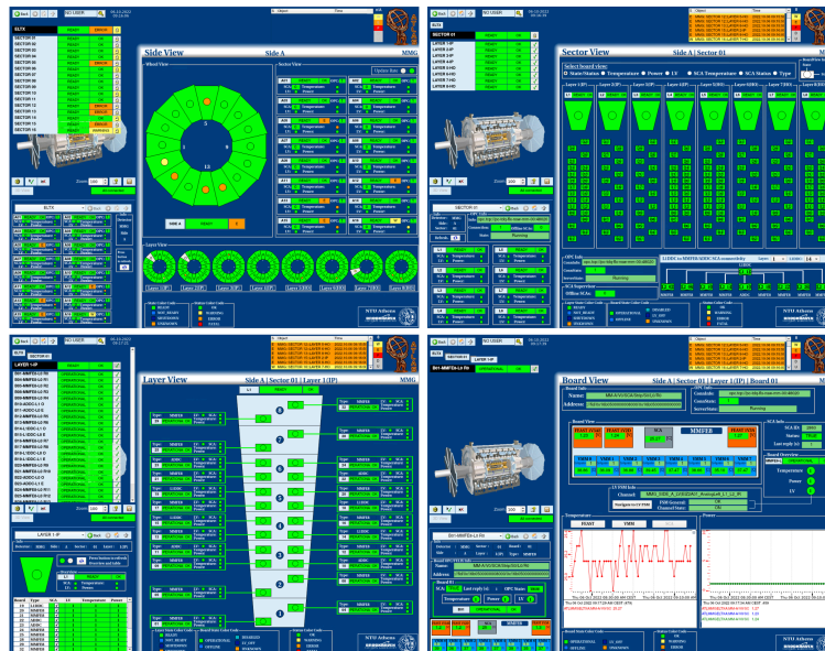
Figure 4: The DCS FSM and panels for the NSW Electronics monitoring.
