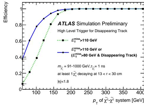
**Figure 4:** The efficiency of the disappearing track trigger for a chargino pair system as a function of transverse momentum. The disappearing track trigger shown as the solid blue line has a lower  $E_T^{\text{miss}}$  threshold of 80 GeV compared to the standard trigger with a threshold of 110 GeV [11].
