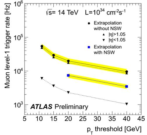
**Figure 5:** Estimation of the Run 3 L1 trigger rates, extrapolated for  $pp$  collisions at  $\sqrt{s} = 14$  TeV, as a function of the  $p_T$  threshold [5].
