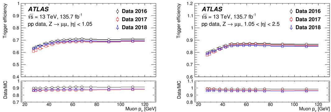
**Figure 4:** Efficiency of passing either the HLT\_MU26\_ivarmedium or the HLT\_mu50 trigger as a function of the offline-reconstructed muon  $p_T$  in the barrel (left) and endcap (right) regions [3].
