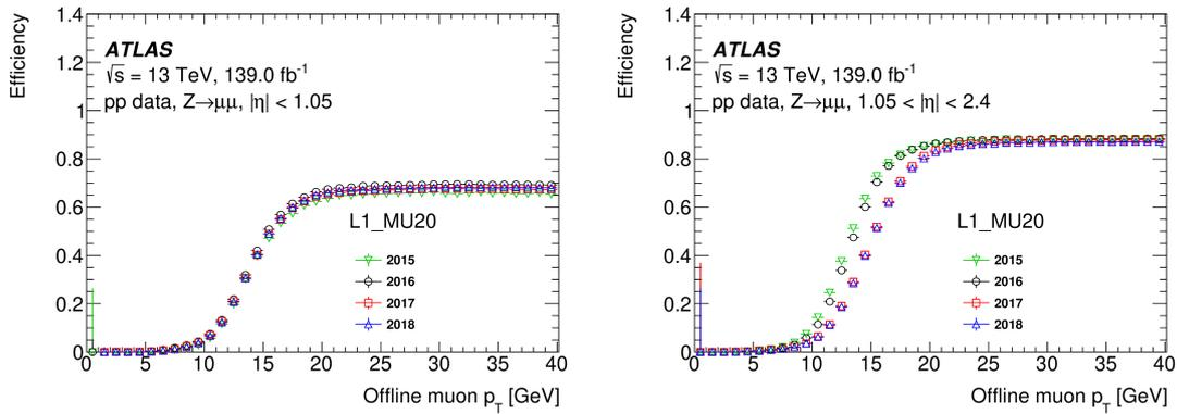
**Figure 3:** Efficiency of the L1\_MU20 trigger as a function of the offline-reconstructed muon  $p_T$  in the barrel (left) and endcap (right) regions [3].
