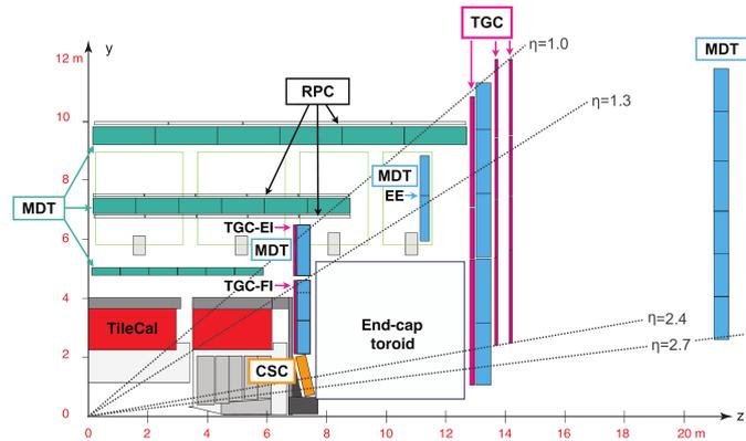
**Figure 2:** A quarter-section view of the Muon Spectrometer in a plane containing the beam axis [3].
