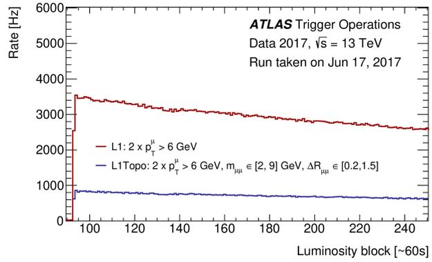
**Figure 1:** L1 trigger rate, as measured during a 2017 run, without (red) and with (blue) the L1Topo requirement. The rate is reduced by approximately a factor of 4 at the cost of a 12% reduction in the HLT efficiency with respect to offline reconstruction [3].
