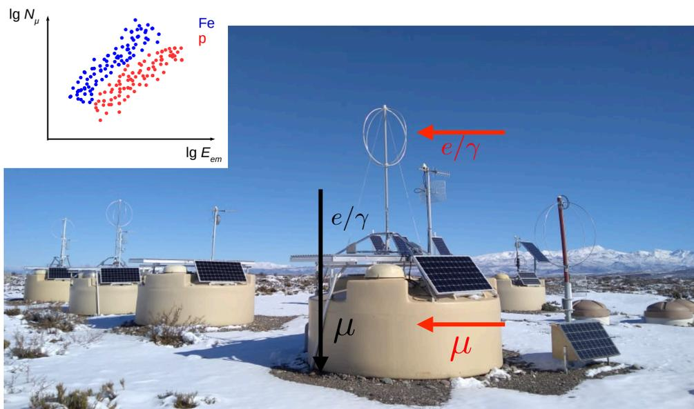
**Figure 1:** Prototype Surface Detector stations of the upgraded Pierre Auger Observatory. The hybrid detection capabilities are illustrated: the muonic component is measured with the water-Cherenkov detectors, while the electromagnetic component is measured with the Scintillator Surface Detector (installed above the water-Cherenkov detector) for vertical showers and with the radio antennas for inclined showers.
