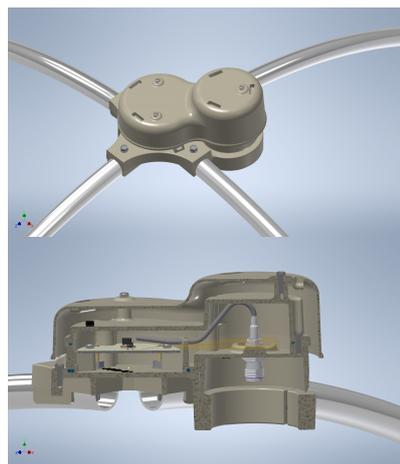
**Figure 3:** Schematic illustration of the top of the SALLA antenna.
