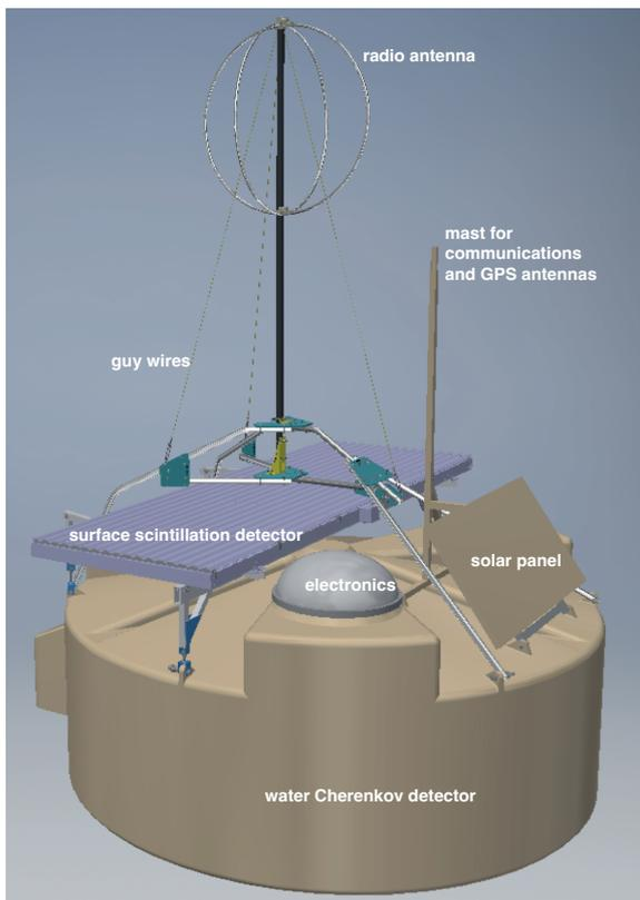
**Figure 2:** Schematic view of an upgraded station of the Surface Detector array. The main components are indicated: the water-Cherenkov detector, the Scintillator Surface Detector, and a radio antenna. A solar panel provides energy for the local electronics. Time synchronization is obtained via the GPS antenna and communications to the central data acquisition system is conducted via wireless communication.
