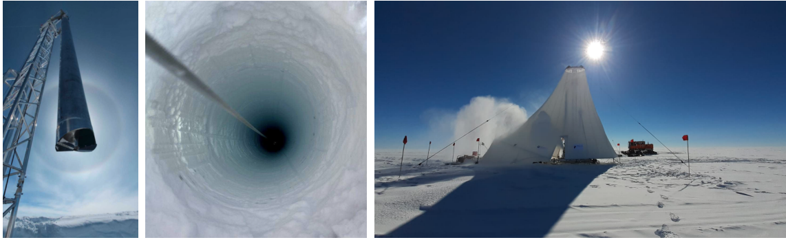
Figure 4: The British Antarctic Survey’s BigRAID auger drill used to drill 11-inch diameter holes ( center ) to a depth of 100 m. The tent ( right ) was added in the 2022 drilling season.
