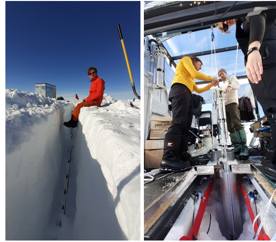
Figure 3: Layout of the hybrid RNO-G station with LPDA antennas deployed in shallow trenches, and V-Pol and H-Pol antennas installed in the deep bore-holes. The deployment process for the shallow and deep component, respectively, is illustrated above.
