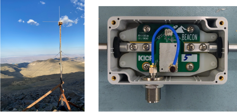
Figure 2: Left: One of the BEACON prototype crossed-dipole antennas. The antenna is elevated 13 ft off the ground and is pointed towards the valley to the East. Right: The BEACON active balun consisting of a 4:1 transformer fed into a 50 \Omega LNA, housed in a Polycase enclosure. The antenna tines pass through water-tight grommets and are connected directly to the front-end board. Pictures sourced from [7].
