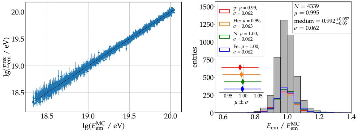
**Figure 3:** *Left:* Scatter plot of the reconstructed electromagnetic shower energy as a function of the true energy for all showers passing our selection. The dashed line indicates the diagonal. *Right:* Histogram of the ratio of the reconstructed electromagnetic shower energy over the true electromagnetic energy. The colored lines indicate the distribution for a particular primary. The legend displays the resolution and bias.
