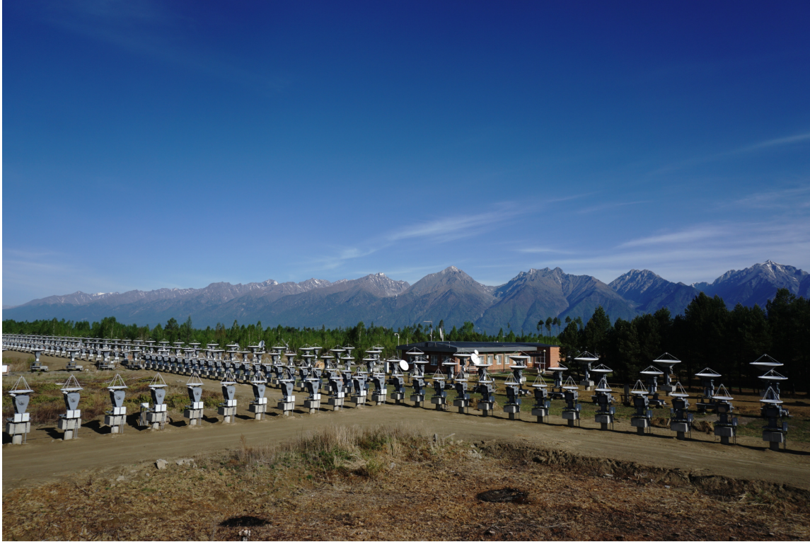
Figure 1: The central part of SRH antenna arrays. The back row is the 3-6 GHz array, which has 3-meter dishes and 9.8 meters spacing between the antennas, middle row is the 6-12 GHz array with 2-meter dishes and spacing of 4.9 meters, and the smallest antennas are the 12-24 array with 1-meter dishes, whose center has 2.45 meters spacing.
