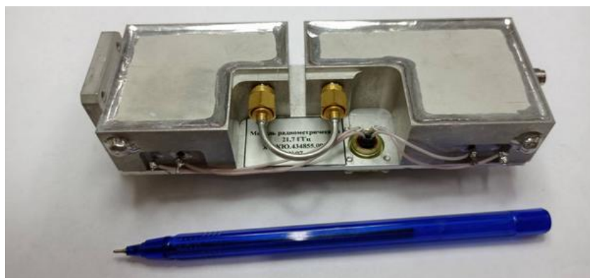
Figure 3: Radiometric module F_0 = 22.25 \text{ GHz} , B = 2500 \text{ MHz} .
