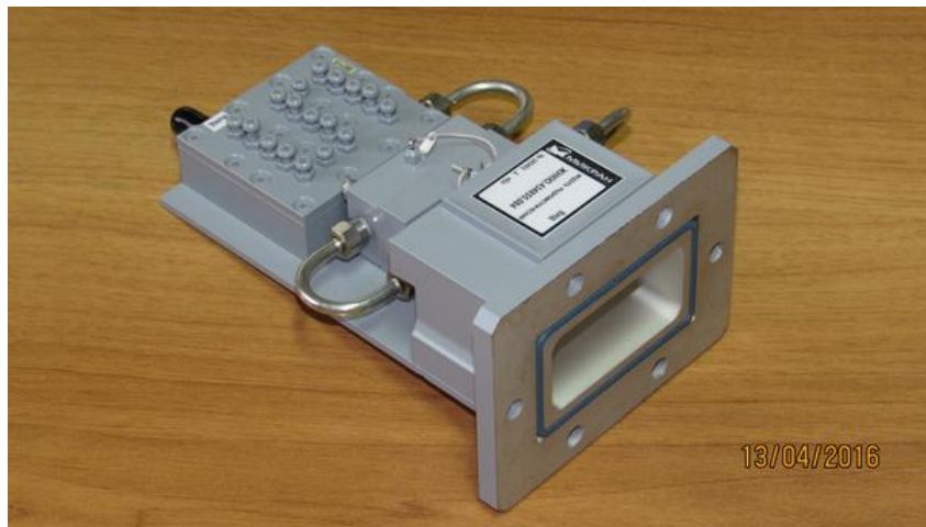
Figure 2: Radiometric module F_0 = 4.7 \text{ GHz} , B = 600 \text{ MHz} .
