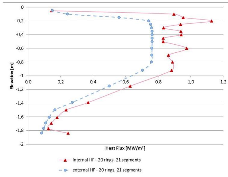
Figure 8: Bounding curves of maximal heat flux values reached in the segments
