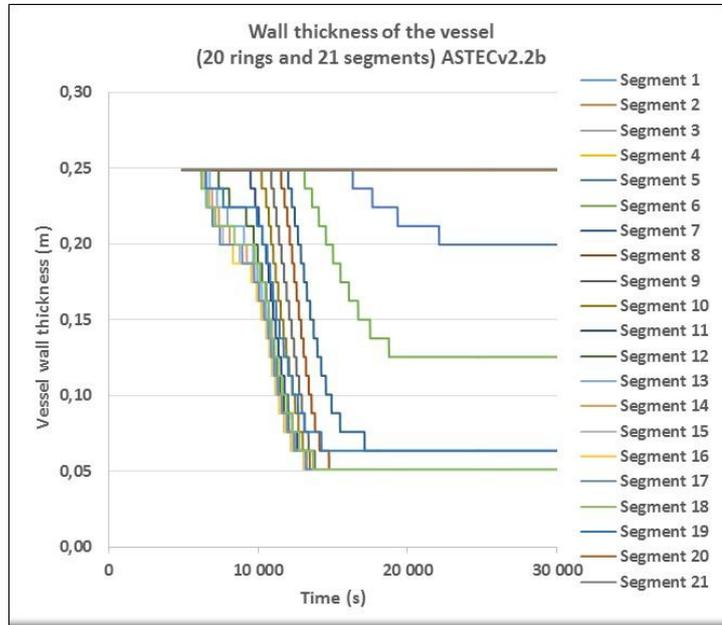
Figure 9: Vessel wall thickness in segments
