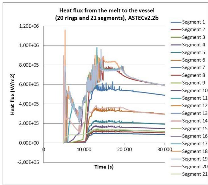
Figure 6: Heat flux from the corium pool to the internal surface of the LP vessel
