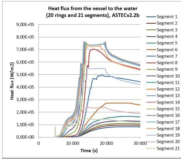
Figure 7: Heat flux from the external surface of the LP vessel to the outside cooling water
