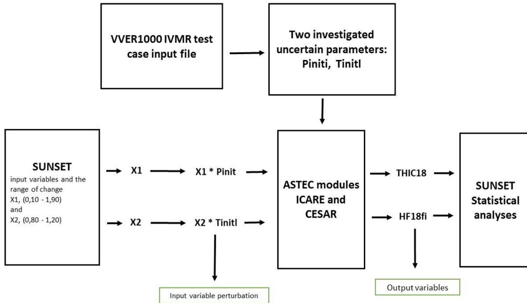
Figure 2: SUNSET/ASTECv2.2b IVMR WWER1000 test case example
