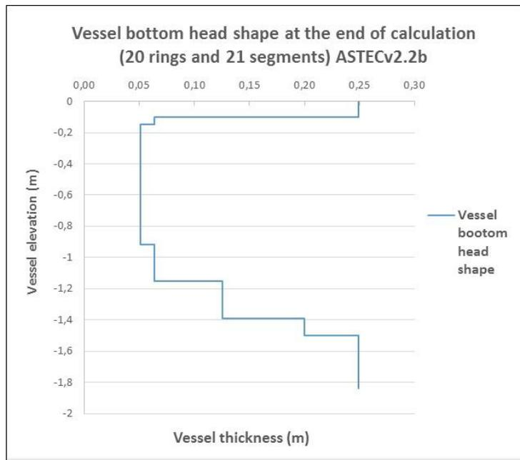
Figure 10: Vessel LP shape at the end of calculation
