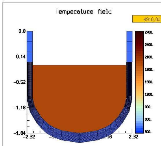
Figure 4: Lower plenum geometry and the corium in it at the beginning of the calculation
