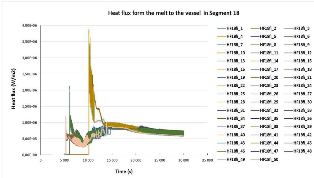
Figure 12: Heat flux from the melt pool to the LP vessel wall (Segment 18)
