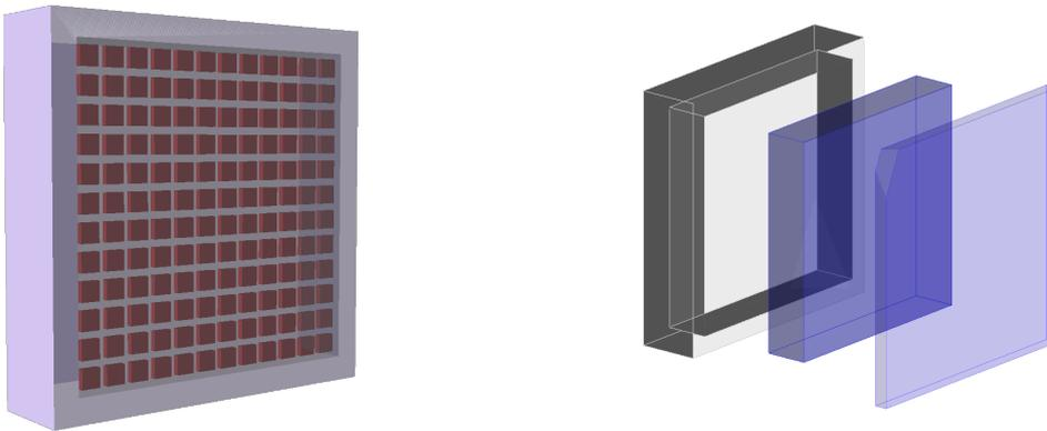
**Figure 1:** Typical scintillator simulation targets. Left: Scintillator with the attached SiPM sensitive detector matrix. Right: Exploded view of the scintillator - reflective case, crystal, glass cover for hygroscopic protection.
