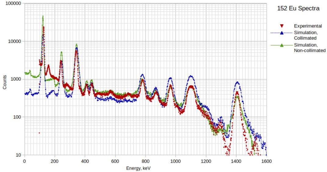
**Figure 6:** Simulated and experimental data of  $^{152}\text{Eu}$  spectra from an in-house readout system for a comparable number of events.
