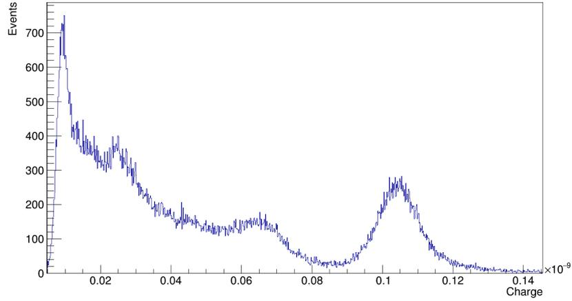
**Figure 5:** Experimentally measured  $^{137}\text{Cs}$  energy spectrum using the 4-column readout from AiT. The spectrum measurements are very close to the expected resolution.
