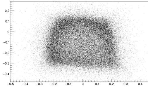
**Figure 4:** Experimentally measured  $^{137}\text{Cs}$  position resolution for the 4-channel readout from AiT. The position measurements using this summation scheme (shown in units of SiPM pixel size) are too crude to be of experimental value.
