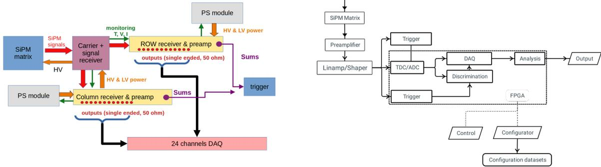
**Figure 3:** Left: Data acquisition using AiT instruments' channel summing technologies. Right: Schematic of Individual Readout Based on Amplitude-to-Time transformation and measurements of ToT and ToA using an FPGA-based TDA algorithms.
