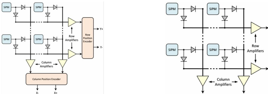
**Figure 2:** Channel-summing readout schematic of AiT Instruments' modules. Left: 4-channel summation ([6]). Right: Row-and-Column summation. ([7]).
