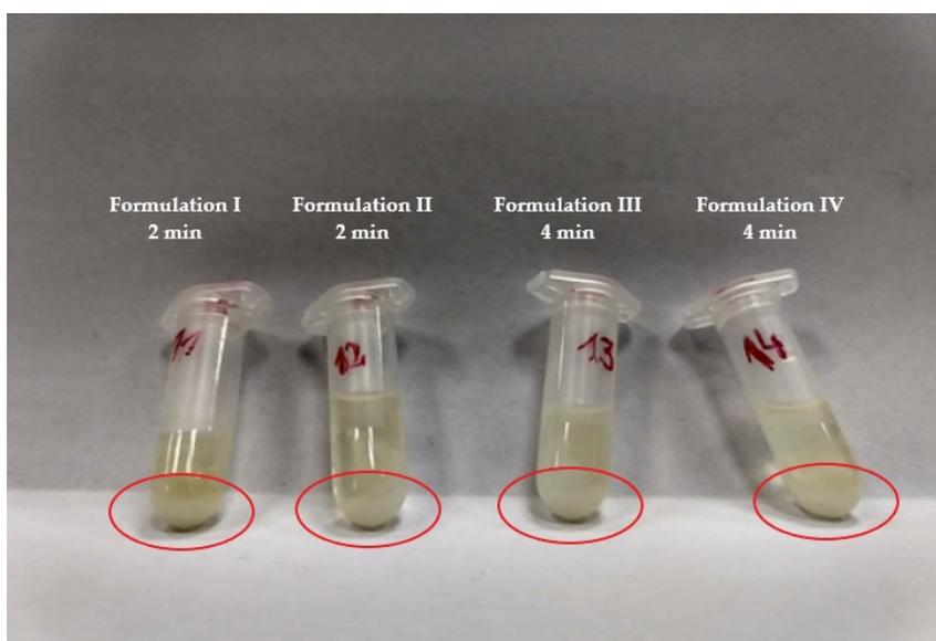
**Figure 4:** Complete phase separation after centrifugation at 3000 rpm.
