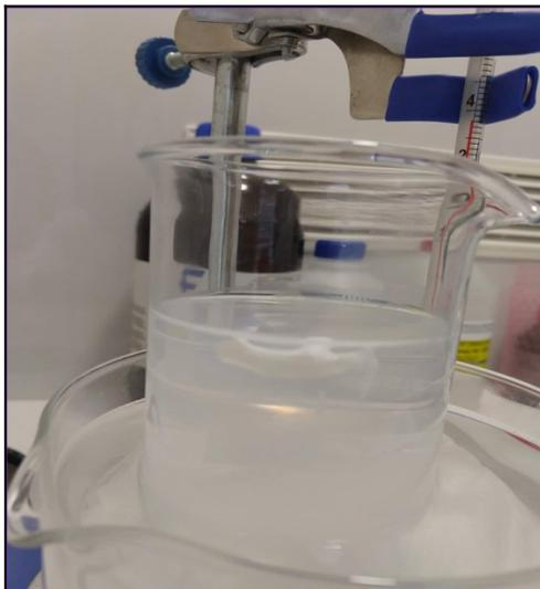
**Figure 3: Self – emulsification time experimental setup**
