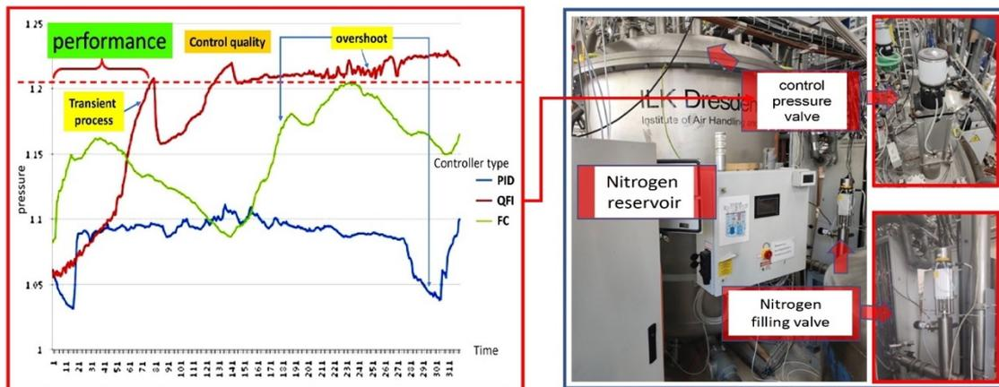
**Figure 10:** Pressure P13 when filling with nitrogen in the mode of cooling current leads and screens
