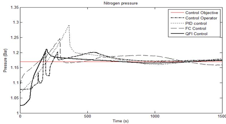
**Figure 8:** Pressure in the nitrogen collector with nitrogen cooling
