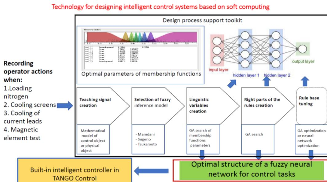
**Figure 7:** ICS design technology and interaction with Tango-Control
