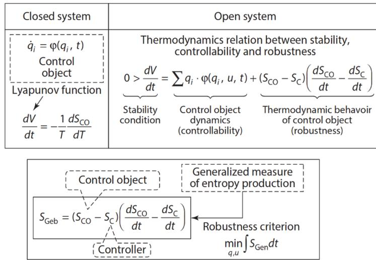
**Figure 2:** Thermodynamic criterion of distribution of quality of robust control
