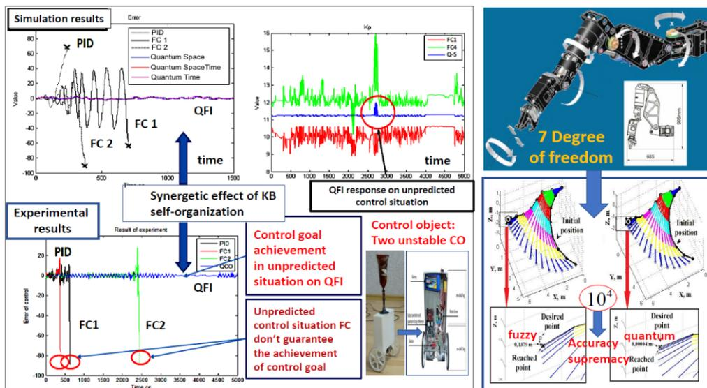
**Figure 3:** The experiment of control in unexpected situations for an object "cart-double pole" and a 7 degrees of freedom redundant manipulator
