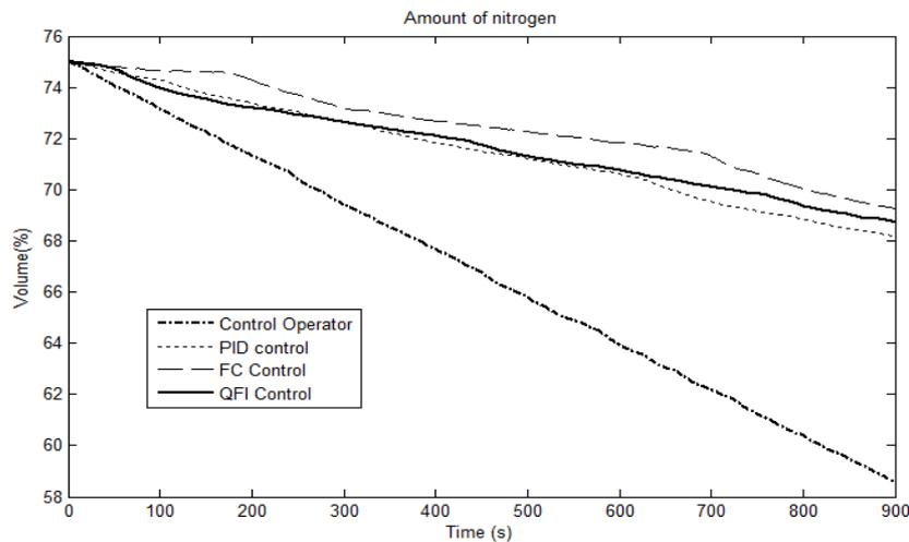
**Figure 9:** Nitrogen consumption in the storage tank
