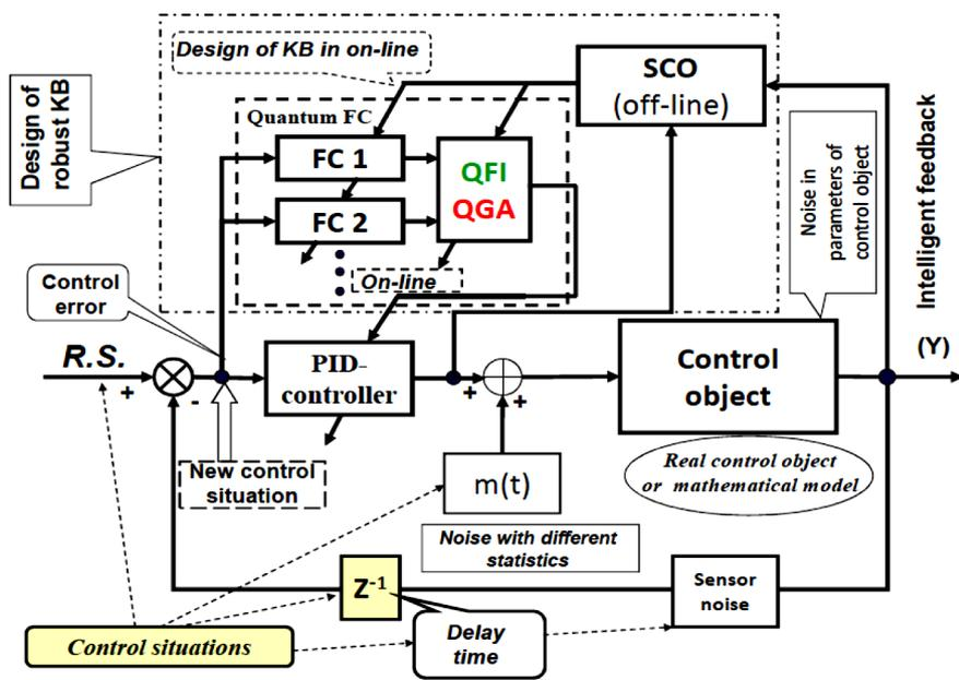
**Figure 1:** Structure of a robust QFI-based self-organized ICS
