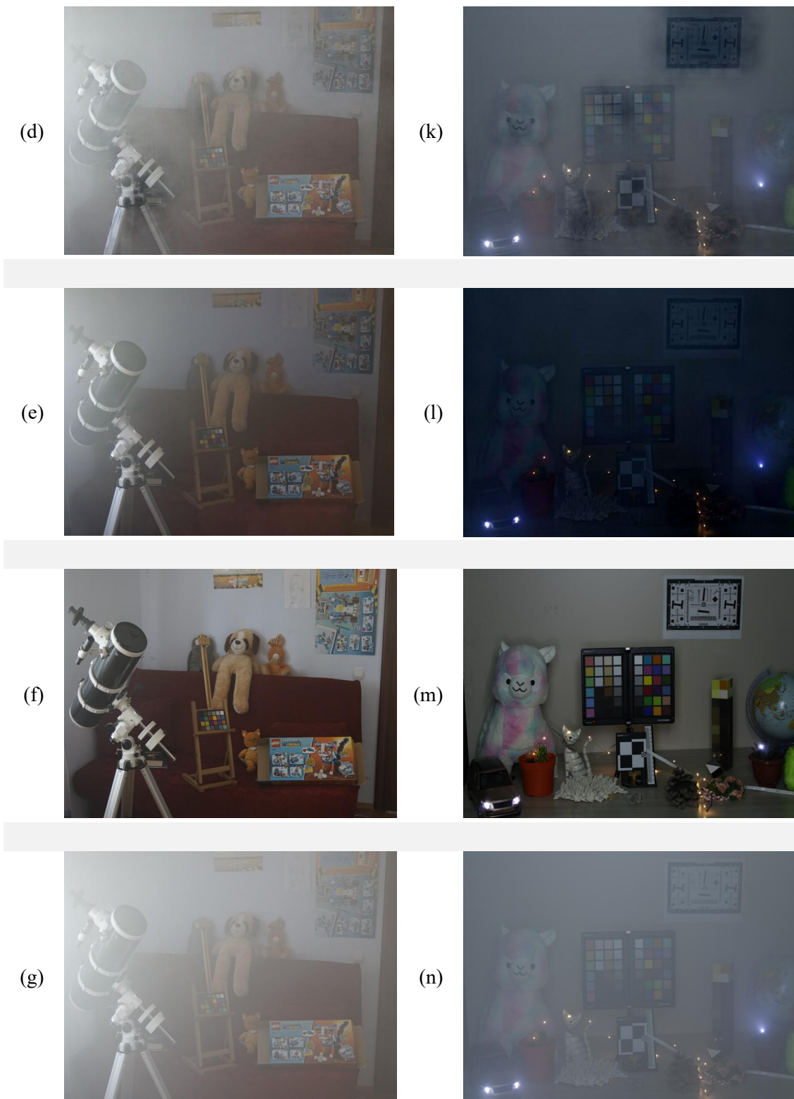
Figure 3: Results of haze removal from images (g) (file 34_indoor_hazy.jpg from the i-haze dataset) and (n) (file stage-2_frame-24_light-2_h3.jpg from the night-haze dataset). Images (a)-(e) correspond to the results of processing (g) by Berman methods et al, Dhara et al, He et al, Qin et al, Zhu et al; (h)-(l) correspond to similar results of image processing (n); (f) – ground truth for image (g); (m) – ground truth for the image (n)
