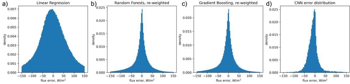
**Figure 4:** Error distribution figures for: a) Linear Regression, b) Random Forests (re-weighted), c) Gradient Boosting (re-weighted), d) CNN
