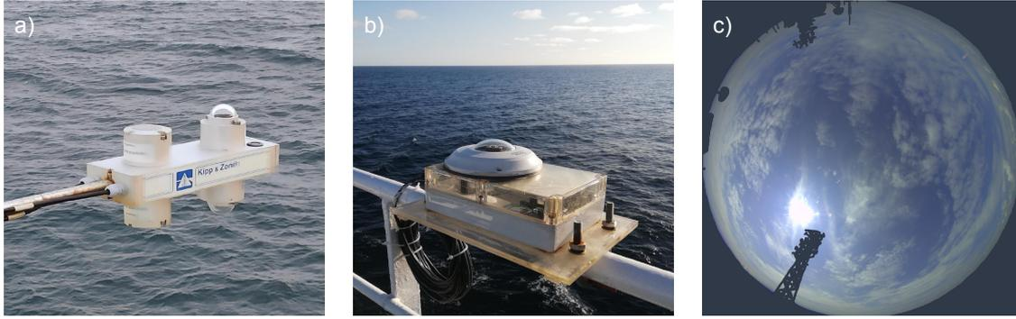
**Figure 1:** Equipment we use to collect the data, and an example of all-sky optical imagery over the ocean: a) radiometer Kipp&Zonen CNR-1; b) cloud-camera «SAIL cloud v.2»; c) all-sky photo with mask.
