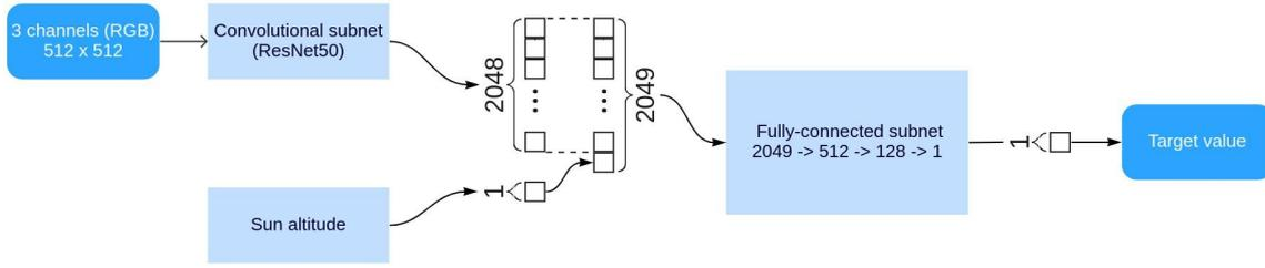
**Figure 2:** Architecture of a CNN we exploited in our study. Here, with numbers, we present the shapes of input data or activation maps.
