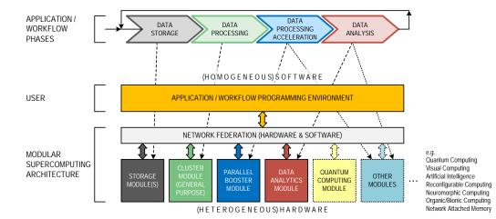
Figure 2: Modular Supercomputing Architecture.
